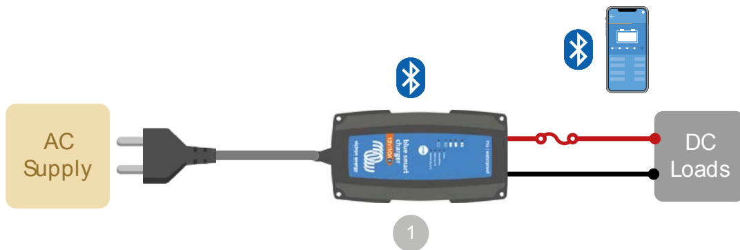
Battery charger used as a power supply.
