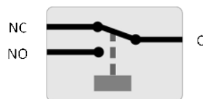
Relay configuration (not energised).
